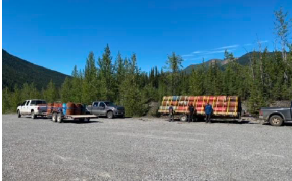
PHOTO 7 - Fuel drums were loaded onto flat deck trailers at the Mile 113 staging for transport to the Fort Nelson dump. Photo: S. Neudorf, August 2022
